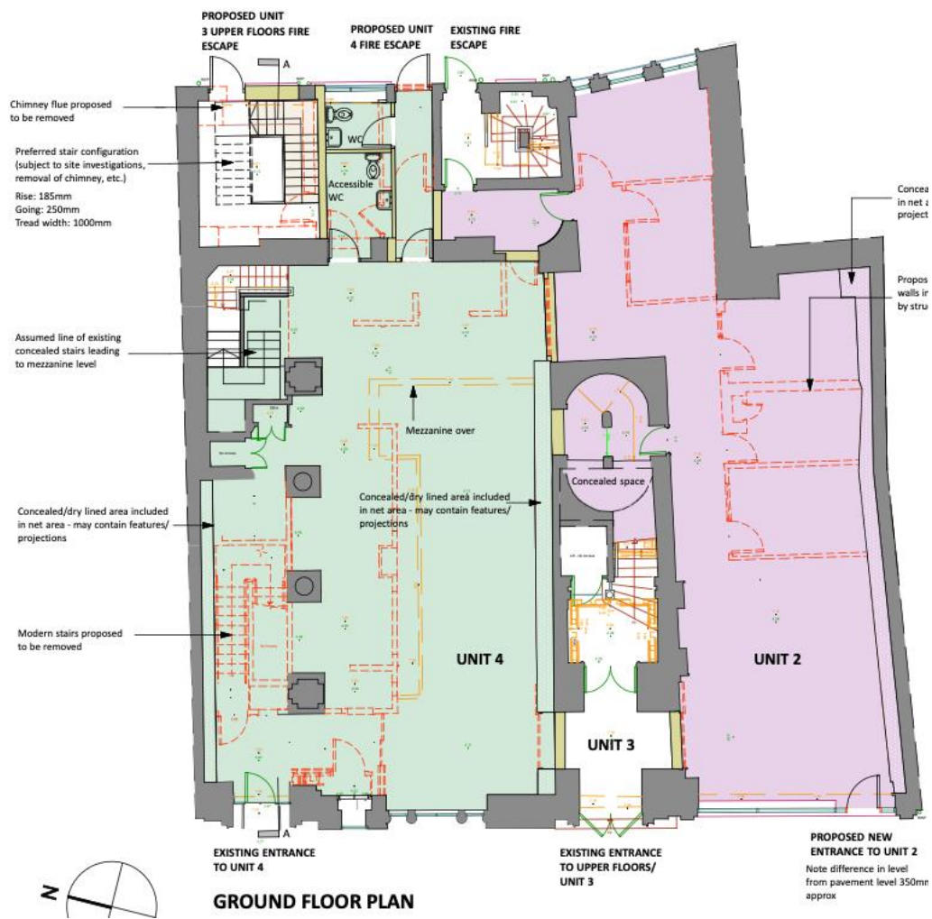
Figure 9 – Proposed Ground Floor Plan for the Initial Pre-Planning Stage
